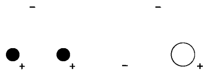
FIGURE 8-7. Comparison and contrast. Left: Two protons and an electron forming the hydrogen molecule ion of chemistry. (A proton is much more massive than an electron but can be envisioned as occupying less volume.) Right: Two electrons and a positron, forming a polyelectron created by impact of a properly tuned photon (about 4 MeV of energy) on an electron at rest.
